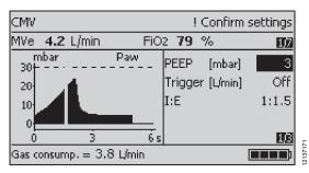
When the PEEP setting is increased above 10 mbar, a message *Confirm PEEP above 10 mbar?* will appear to request confirmation of the change. The PEEP setting can be increased to the desired setting after the message is confirmed with the rotary knob.
