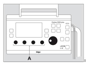
5 Set the control knobs (A) below the display to the required values.
