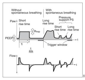
Pressure-controlled ventilation combined with spontaneous breathing throughout the respiratory cycle and variable Pressure Support at CPAP level.
