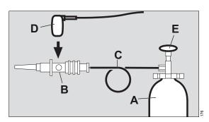
2 Connect the test gas cylinder (A) and the cuvette (B) of the calibration set to the hose (C).
