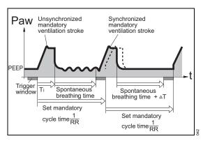
VC-SIMV provides a combination of mandatory ventilation and spontaneous breathing. It enables the patient to breathe spontaneously, with the mechanical mandatory breaths providing minimum ventilation. The minimum ventilation is controlled by the two set values of the tidal volume *VT* and respiratory rate *RR* and is determined from the product of VT x RR.
