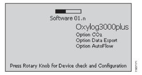
The Oxylog 3000 *plus* performs a selftest. The selftest will be completed in approximately six seconds.
