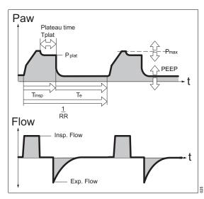
Volume-controlled ventilation with fixed mandatory minute volume MV, which is set with tidal volume *VT* and respiratory rate *RR*.
