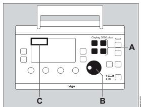
Press the appropriate ventilation mode key (A) for approximately 3 seconds.
