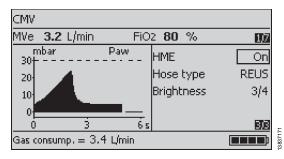
When **HME - ON** is selected, the flow sensor expects an expiration gas temperature of 35 °C and a relative humidity of 0 %.
