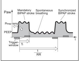
As with VC-SIMV, the time pattern is set using the basic setting parameters of respiratory rate *RR* and ventilation time ratio *I:E* or inspiratory time *Ti*.
