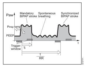
The PC-BIPAP ventilation mode is a pressure controlled / time-cycled ventilation mode, in which the patient can always breathe spontaneously. PC-BIPAP can be described as a time-cycled alternation between two CPAP levels.
