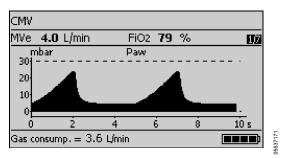
Curve window showing the airway pressure curve Paw.
