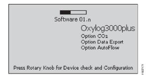
2 Press the rotary knob (B) to confirm, before the black progess bar is complete. The start-up screen appears:
