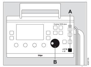
To switch the device ON, briefly press the () key (A).
