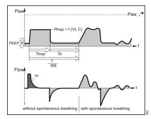
AutoFlow (AF) delivers the set tidal volume *VT* using a decelerating flow pattern to achieve the lowest peak airway pressure possible. The Oxylog 3000 *plus* determines the pressure required to deliver the set tidal volume *VT* based on lung characteristics such as resistance and compliance relationships, and the patient's spontaneous breathing demand.
