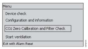
3 Select CO2 zero calibration and filter check in the start-up menu and confirm.
