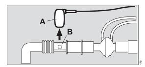
Remove the CO<sub>2</sub> sensor (A) from the cuvette (B).
