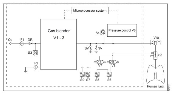
The various pneumatic actuators in the Oxylog 3000 *plus* are controlled by the microprocessor system via digitized electrical signals.
