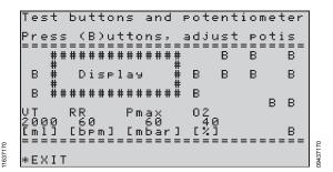
The operating elements on the front panel are displayed schematically on the screen.
