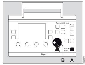
1 To switch the device OFF, hold down the key (A) for approximately 3 seconds.
