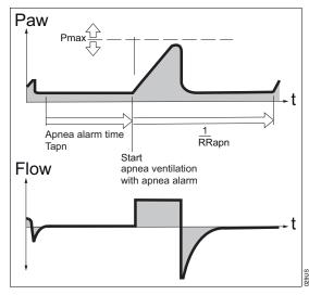
Apnoea back-up ventilation is only applicable when using the SpnCPAP mode. In the event of an apnoea, the ventilator will automatically activate volume-controlled mandatory ventilation - (VC-CMV).
