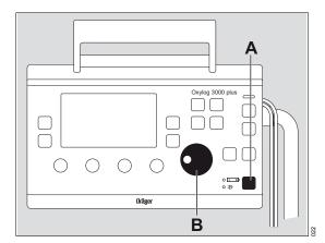
1 To switch the device ON briefly press the key (A).
