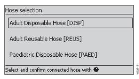
Select the connected hose type, as seen in the above graphic, by rotating the rotary knob (B) and confirm by pressing the rotary knob (B). The ventilator now automatically begins ventilation with the default settings.
