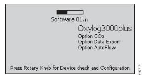
2 Press the rotary knob (B) to confirm, before the black progress bar is complete.
