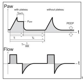
In this mode only mandatory volume controlled strokes are delivered to the patient. The ventilation pattern is specified by the settings for tidal volume *VT*, respiratory rate *RR*, ventilation time ratio *I:E* or inspiratory time *Ti* and *PEEP*.
