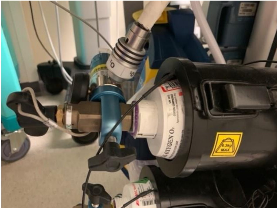
2 E cylinder with regulator in situ on the old trolley
