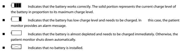
The capacity of the internal battery is limited. If the battery charge is too low, a technical alarm will be triggered and the message [Low Battery] or [Battery Depleted] displayed. At this moment, apply AC/DC power to the patient monitor. Otherwise, the patient monitor will power off automatically before the battery is completely depleted.
