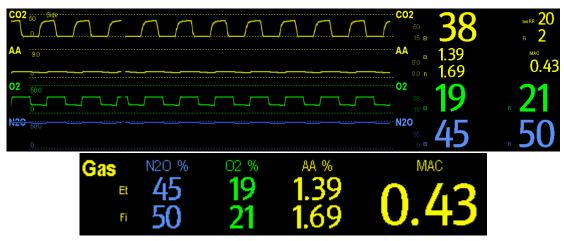
The AG module can send waves and numerics for all measured anesthetic gases for display on the monitor, including:
